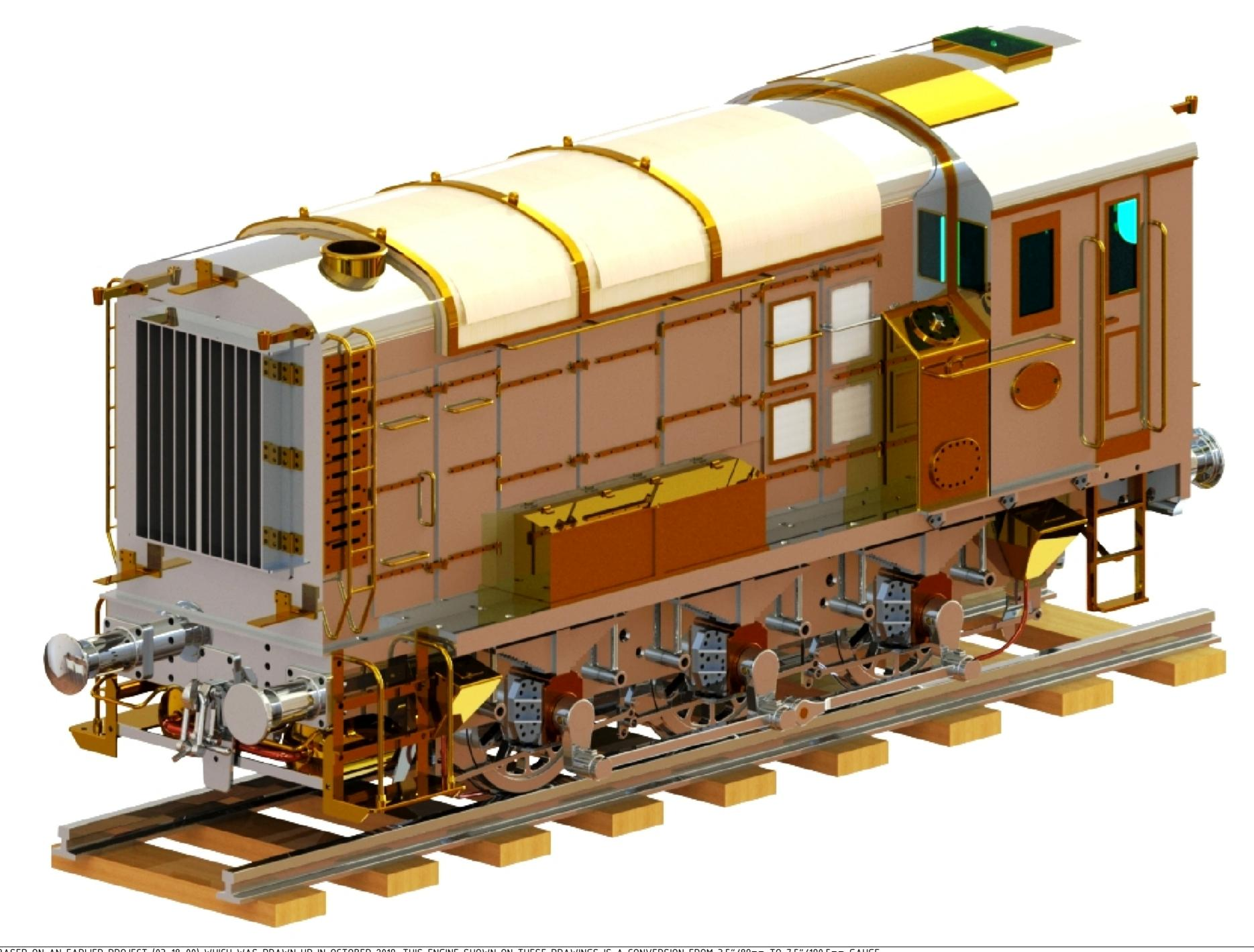
NOTES: THIS ENGINE IS BASED ON AN EARLIER PROJECT (03-18-00) WHICH WAS DRAWN UP IN OCTOBER 2019. THIS ENGINE SHOWN ON THESE DRAWINGS IS A CONVERSION FROM 3.5"/89mm TO 7.5"/190.5mm GAUGE
