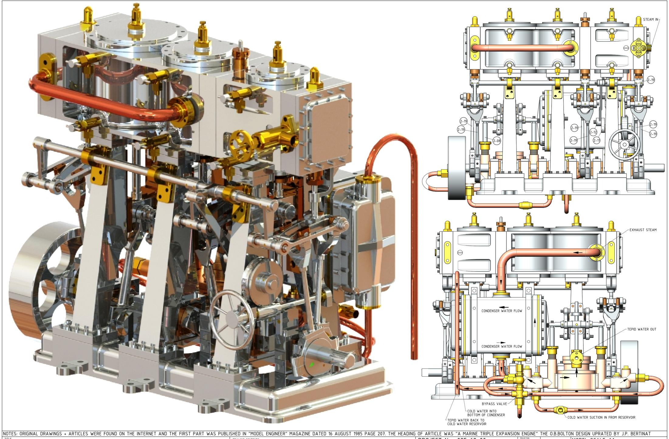
A MODEL OF A MARINE TRIPLE EXPANSION STEAM ENGINE (BORE: HP=44, IP=64, LP=90 S=64mm)
