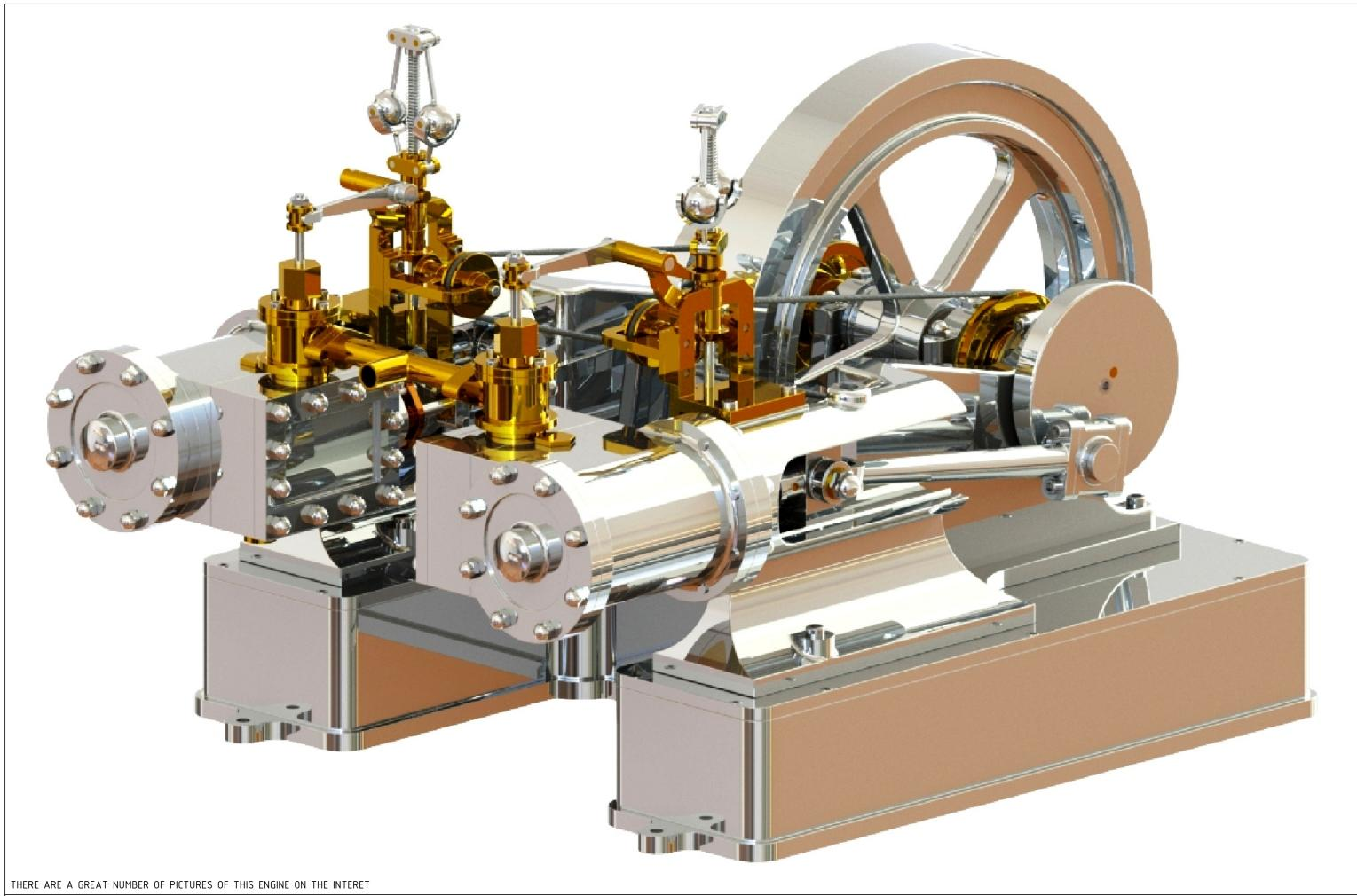
NOTES: FOUND ORIGINAL DRAWINGS ON THE INTERNET. THE DRAWING TITLE WAS "DOUBLE TANGYE TYPE MILL ENGINE" BY EDGAR T WESTBURY. THE ENGINE SHOWN ON THESE DRAWINGS IS APPROXIMATELY 1.5 TIMES THE ORIGINAL SIZE
