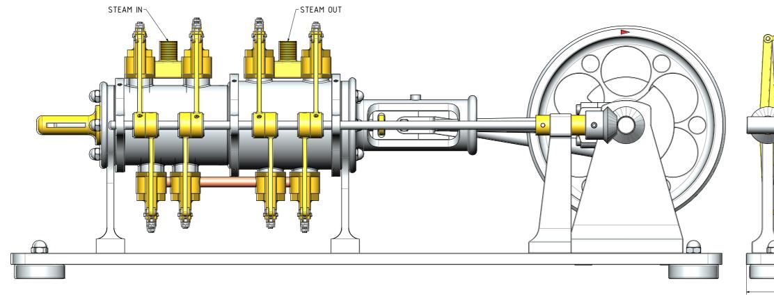
NOTES: THIS ENGINE IS LOOSIE BASED ON AN ENGINE OF WHICH PHOTOGRAPHES WERE PUBLISHED IN A DUCTH MODEL MAGAZINE. NO DRAWINGS WERE ISUEED OR SHOWN TO DESIGN THIS ENGINE. THIS DESIGN IS BY JDW. GENERAL ARRANGEMENT EXP. DUPLEX COMPOUND STEAM ENGINE
