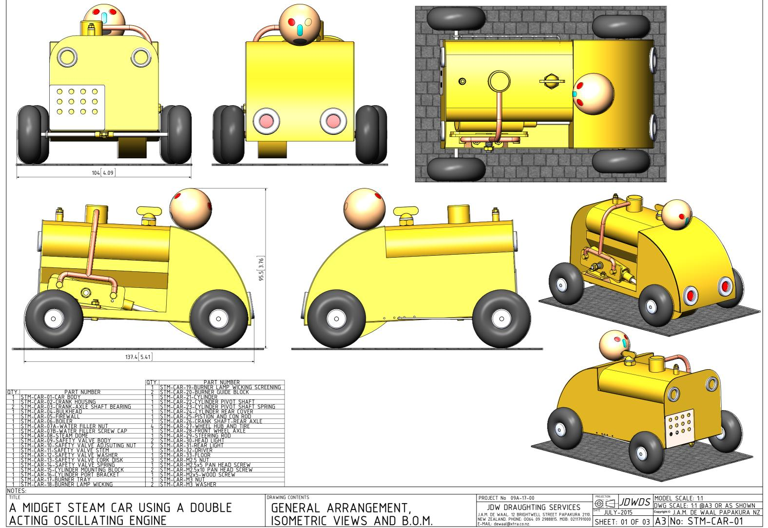
A MIDGET STEAM CAR USING A DOUBLE ACTING OSCILLATING ENGINE
