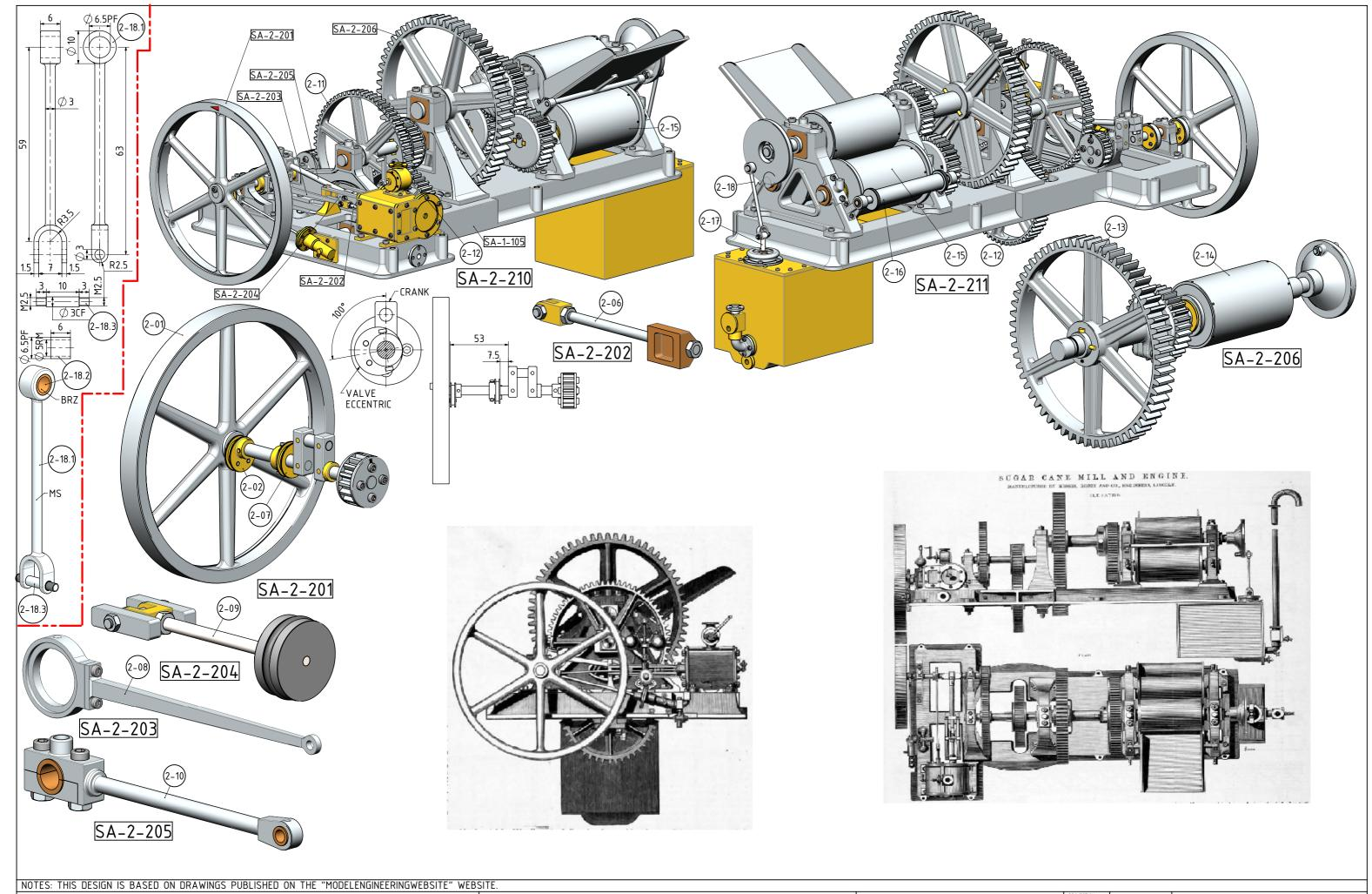
A MODEL OF A SUGAR CANE MILL AS MANUFACTURED BY MESSERS. ROBEY&CO PARTS AND ASSEMBLIES ORIGINAL DRAWINGS
