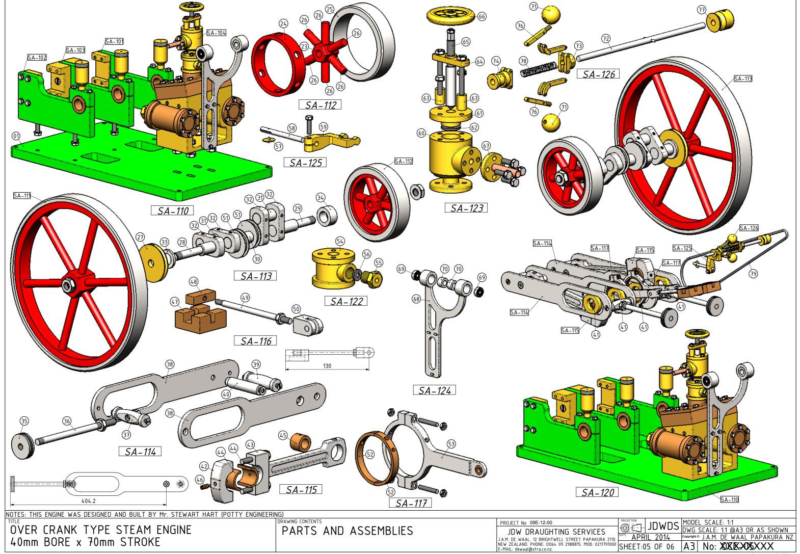
OVER CRANK TYPE STEAM ENGINE 40mm BORE x 70mm STROKE
